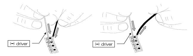
Inserts the end of lead wire while pressing the button with (-) driver.
