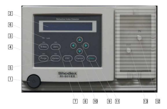
Fig. 5.1 Front panel of **Shodex** RI-501EX
